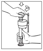
Replace TOP by engaging lugs and rotating 1/8 turn clockwise. MAKE CERTAIN TIP IS TURNED TO THE LOCKED POSITION. VALVE MAY NOT TURN ON IF TOP IS NOT FULLY TURNED TO THE LOCKED POS
